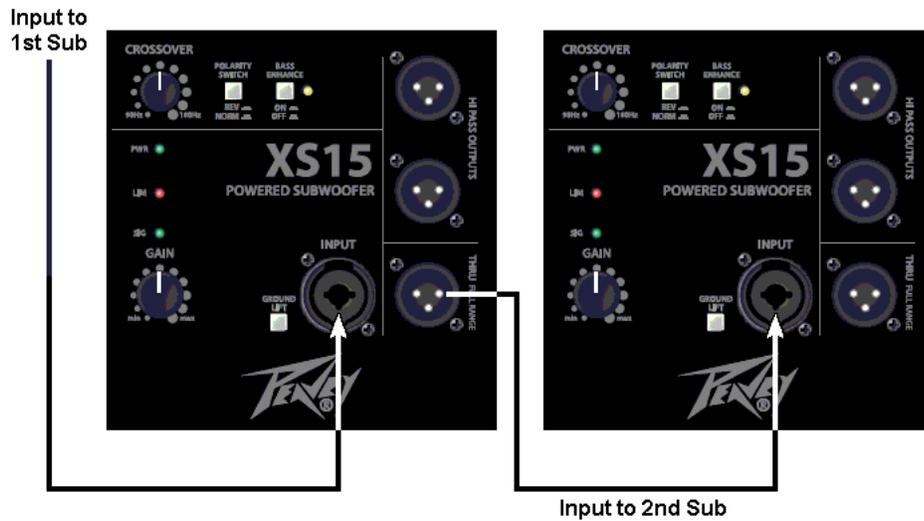
The powered loudspeaker system shall have a frequency response from 47 Hz to 180 Hz with the Crossover knob turned all the way CW, and from 47 Hz to 90 Hz with the Crossover knob turned all the way CCW, at the - 6 dB points. The peak SPL with inaudible distortion shall reach 127 dB with music as a source, when measured at a distance of 1M and driven to full output capacity. The system shall utilize a premium 15" heavy-duty woofer in a vented enclosure tuned to 50 Hz.
