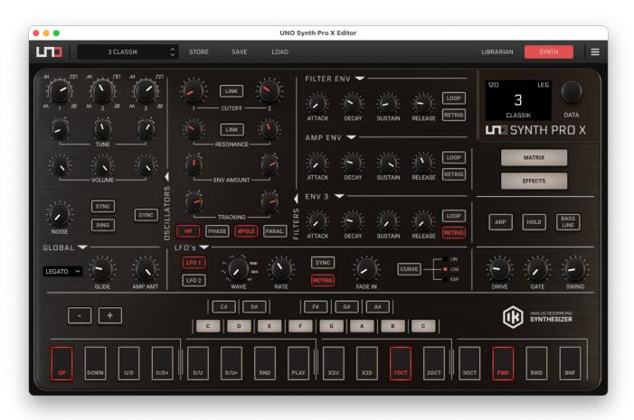
The UNO Synth PRO X Editor is a software utility to help you edit and manage the presets of your hardware synthesizer. It works both standalone and as a plug-in for use within a DAW, so you can edit and even automate your UNO Synth PRO X just like a software synthesizer, but with all of the sonic mojo of a real analog hardware synth.
