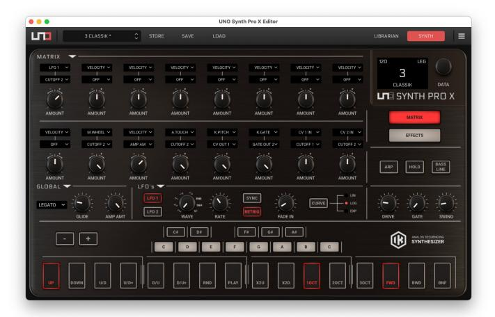
The UNO Synth PRO X has a 16-part Modulation Matrix where you can assign a Source to modulate a Destination by a fixed amount. Click the Matrix tab to view and edit the 16 available modulation routes.
